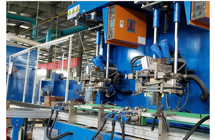
Automatic through - wall welding
