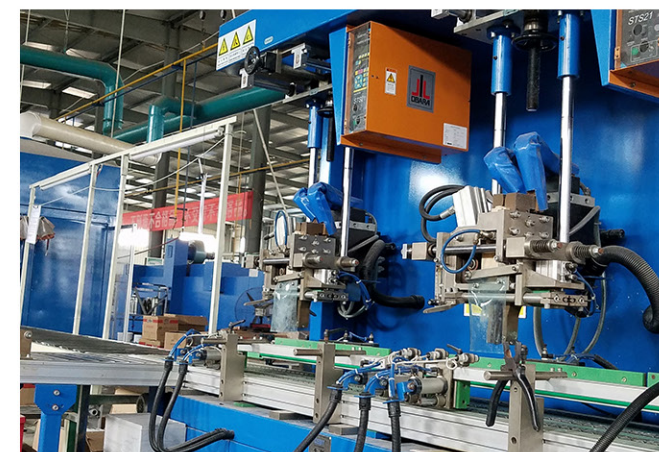
Automatic through - wall welding
